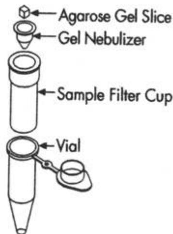
6. Place the gel slice in the Gel Nebulizer and seal the device with the cap attached to the vial.
